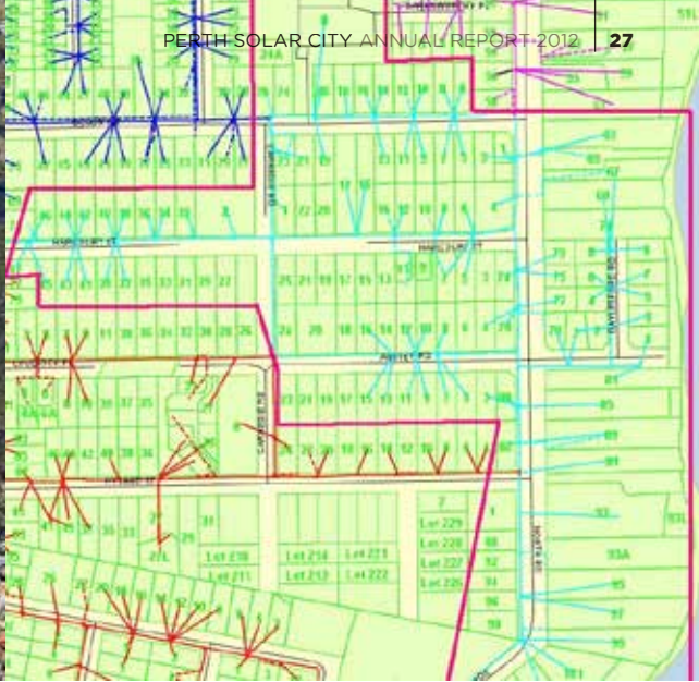
Image 3-L: Anstey transformer distribution LV network
